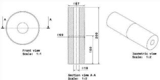
Roller can be considered to be a hollow shaft subjected to torsional load.
